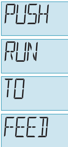
Figure 3-7 PUSH RUN TO FEED Alarm
