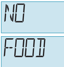
Figure 3-6 NO FOOD Alarm
