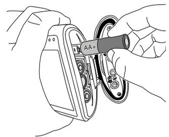
**OR:** If using a rechargeable battery pack, insert it into the pump as shown.
