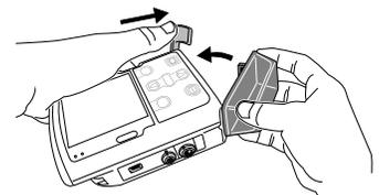
4. Lift the cassette latch into the closed position. A message will briefly appear in the status bar so you can verify the type of cassette you have attached.
