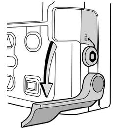
2. Clamp the tubing. Insert the cassette hooks into the hinge pins on the bottom of the pump.
