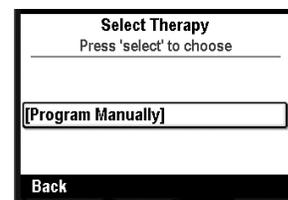
2. On the Select Therapy screen, scroll to the bottom of the therapies until [Program Manually] is highlighted and press **select**.
