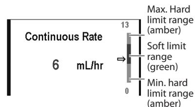
The soft limits (displayed in green) will be the range most commonly used for the protocol, and the hard limits (displayed in amber) extend to the highest and lowest amount that the CADD®-Solis system administrator chooses to allow for the protocol. If the doctor's orders do not match the initial values, they should be edited to match. Editing the parameters above or below the soft limits will result in a screen that requires you to confirm the soft limit override.
