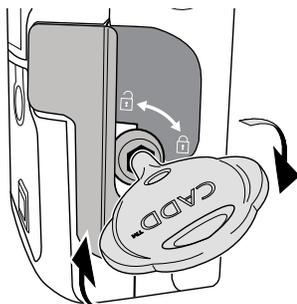
**NOTE:** The cassette **must be locked** in order to start the pump. “Cassette Locked” will appear briefly in the status bar.
