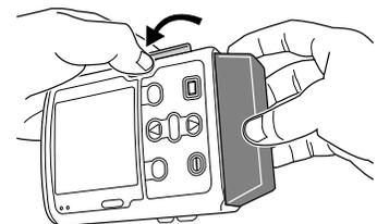
5. Insert the pump key into the cassette/keypad lock and turn clockwise into the locked position.
