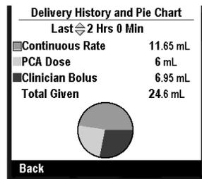
Press **▲** or **▼** to view the time chart in the various time frames. This will provide a quick review of the methods of delivery over the interval selected.
