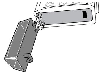
3. Holding the pump in your hands, push down on the cassette latch, and push up on the cassette until it firmly clicks into place.
