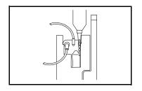
Primary only: Attach an empty container or syringe to the secondary inlet port (syringe shown).
