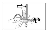
Turn the flow regulator until a drop of fluid is seen in the pumping chamber.
