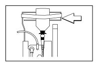
Vial or Syringe: Secure the container to the cassette door using the *optional* container support arm.
