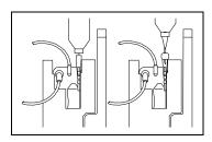
Attach the secondary container to the secondary inlet port (capped port shown on the left, prepierced port on the right).
