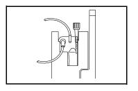
Primary only: Remove the container attached to the secondary inlet port, then cap the port (if appropriate).
