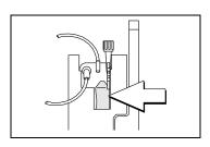
Confirm that the cassette air trap is full of fluid. If air is present, use the backpriming function to expel the air.
