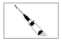
Syringe: Invert the syringe and expel the air (syringe adapter with blunt cannula is shown).
