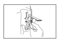
Holding the primed cassette by its fingergrip, slide it into the cassette door guides until it firmly seats in the door. Close the cassette door.
