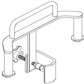
Always mount the tandem carrier (List# 12270-01) to the pole before attaching the pump(s) to the tandem carrier.
