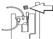
**With cassette door closed: Loosen and remove white cap, then discard. Add secondary tubing or syringe.**
