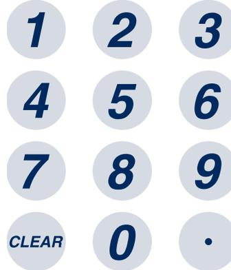
The [CLEAR] key will cause a highlighted numeric field to be cleared in preparation for data entry.
