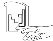
**Insert cassette into door guides. Close the cassette door. Confirm there is no flow and no kinks appear in tubing.**
