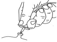
Insert piercing pin into container outlet with a twisting motion.
