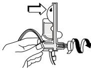
Turn the flow regulator counter-clockwise until a drop of fluid is seen in the pumping chamber.
