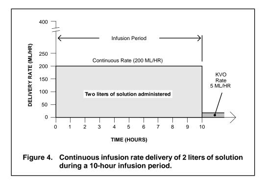
In addition, the CADD-TPN<sup>®</sup> pump can be programmed for gradual changes (tapering) in the infusion rate at the beginning and/or end of the programmed infusion period. Infusion rate changes can be made to occur very slowly or quickly, depending on how the pump is programmed. An example of tapering when two liters of solution are delivered during a 10-hour infusion period is shown in Figure 5. The pump slowly increases the infusion rate in the first
