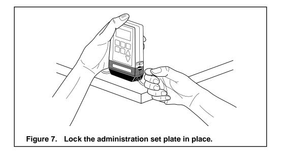
• Gently twist and pull on the set plate to make sure it is firmly attached.
