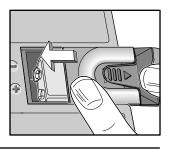
WARNING: If a gap is present anywhere between the battery door and the pump housing, the door is not properly latched. If the battery door becomes detached or loose, the batteries will not be properly secured; this could result in loss of power, nondelivery of drug, and, depending on the type of drug being administered, death or serious injury to the patient.
