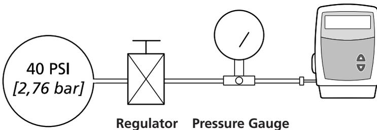
4. Connect the Medication Cassette™ Reservoir outlet tube to the metered pressure source.
