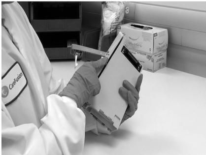
8. Inspect the IUI connectors on each PC unit and module prior to use. Replace any IUI connector with surface contaminants, blue or green deposits, or cracks.
