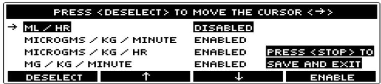
4. Press **Select** button to put the *highlight* on ML / HR. Then press **Enable**. Note how the screen changes.
