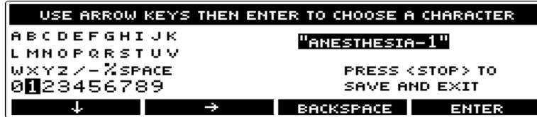
10. When finished naming the template, press the **Stop** key to save and exit. Or press the **Back** key to exit without saving.
