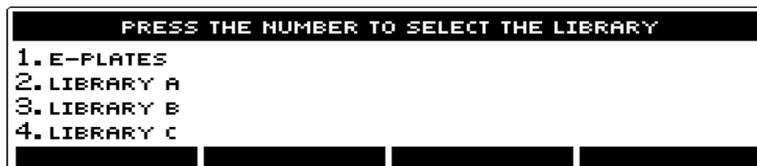
5. Find an unused template, and select it by pressing its **number** button. (You can reuse any template number. The new template *writesover* the old one.)
