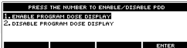
5. When ready press the **Enter** button to set the new Program Dose Display status. Or press the **Back** button to exit without changing the Program Dose Display status.
