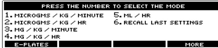
If you press this button, the pump displays the templates in the E-Plates library – and the button is now labeled “MAIN MENU”.
