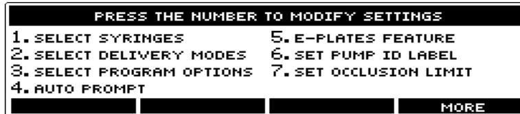
2. Press the **More** button until you locate SELECT PROGRAM OPTIONS. Press its **number** button to call the ENABLE / DISABLE / MOVE screen.
